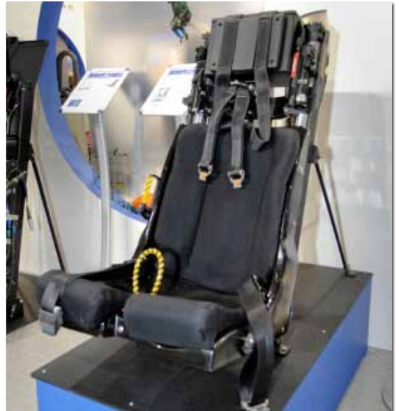
The Mk15B seat has been developed to provide a very lightweight and compact escape system for lightweight aircraft with limited space within the cockpit. Martin-Baker has now equipped the Grob G120 with the Mk15B ejection seat. The Grob G120 is currently the smallest aircraft to be equipped with Martin-Baker ejection seats. The Mk15B seat – weighing just 37kg – is also the first from Martin-Baker to feature a fully composite seat bucket.
