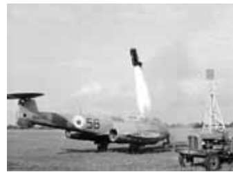
Zero/Zero test from an early Meteor. (Chalgrove)
